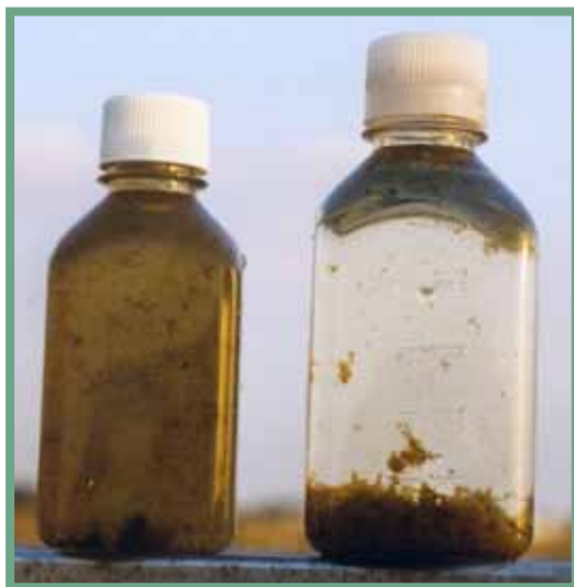
Figure 8: Demonstration of the effect of coagulant and flocculant on Maribrin Farm effluent. (photo STM aquatrade)
