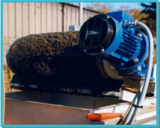
Figure 9: Thickened sludge with belt filter
